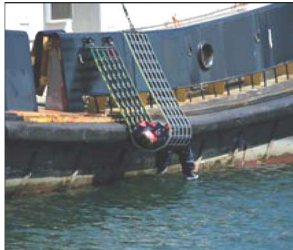
Operating the Jason's Cradle® with high freeboard vessels is no problem using a block and tackle or davit crane system
